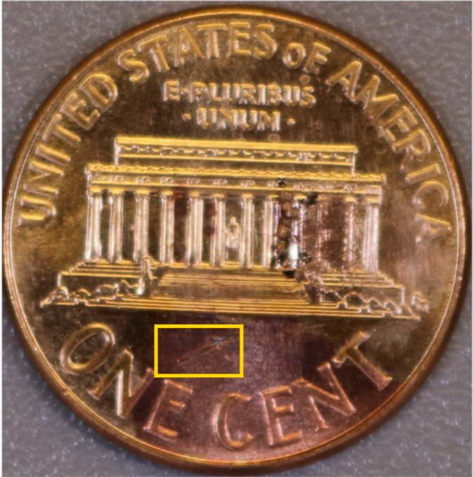
Left: Image of U.S. 1 cent piece (reverse) with gash location shown in yellow box. Below: SEM secondary electron image of portion of gash. Note 50 micron scale bar. Gash exposes zinc underneath copper plate. Energy spectra at bottom show copper and zinc, location of zinc as shown with arrow. Bright area is topographic high of copper plate resulting from gash.
